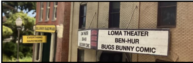
Using the real sign I photo shopped a marquee for the model theater The paper sign was glued to a plastic V shape glued to the front of the building with wire supports
