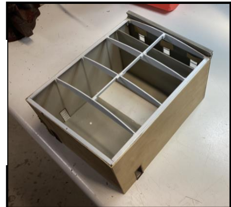
LEFT and RIGHT: The roof arch structure was built from Evergreen .040 sheet styrene, and the bracing are .060 x.170 styrene strips.
