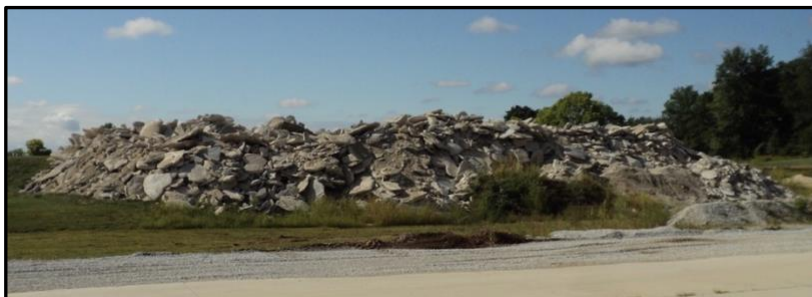
Pictured above and below are two ways excess concrete is recovered. Either used for making large concrete barrier blocks or dumped to be crushed into concrete gravel
