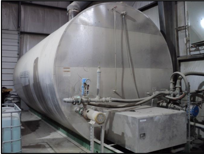
It takes a lot of water to make concrete. A large hot water tank is located inside the plant. The water is fed by the local city water supply
