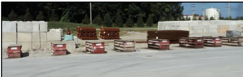
Pictured above and below are two ways excess concrete is recovered. Either used for making large concrete barrier blocks or dumped to be crushed into concrete gravel
