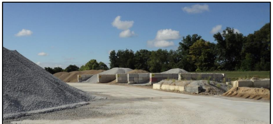
Many types and grades of aggregates are stored in segmented storage bins
